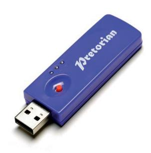
SimplyWorks Receive:2 is functionally identical to Receive but in a smaller form-factor. Which to choose depends on the circumstances and location in which it is going to be used. For example, it may prove beneficial to choose Receive:2 if the SimplyWorks configuration is to be used on more than one computer as it's easier to transport Receive:2 from one computer to another.
