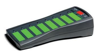
EnvirON® Scanning Remote is a handheld or mountable remote control. Each of its eight large, touch sensitive buttons may be configured to work with any combination of EnvirON® receivers to allow you to control all your appliances from a single remote. For example, some buttons on the Scanning Remote may be configured for TV access while others may be used to turn on a lamp, open a door or close the window.
